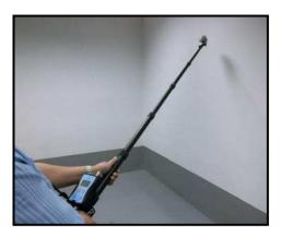
The ERiS2 monitor can be coupled to the telescopic pole, so that the measurements can be made at a distance of 2 meters.
